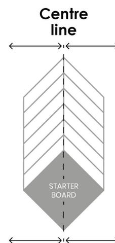
exactly in line with the center line, press the plank down on sub-floor.
