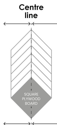
with the top and bottom points aligned with the center line, starting at the nearest wall and following the central line. (Drawing 1.)
